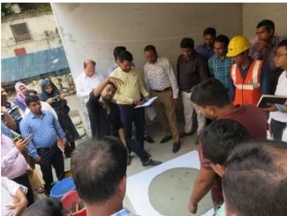
Checking flowability of micro-concrete
